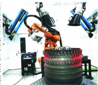
This is local startup AmpTec Industrial Heating's dry ice-blasting facility, which cleans Rolls Royce's aircraft components in an eco-friendly fashion - no industrial chemicals or scrubbing needed.
