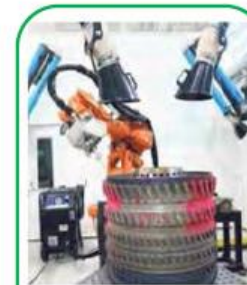
At the Advanced Remanufacturing and Technology Centre, aircraft parts are cleaned using dry ice-blasting.
